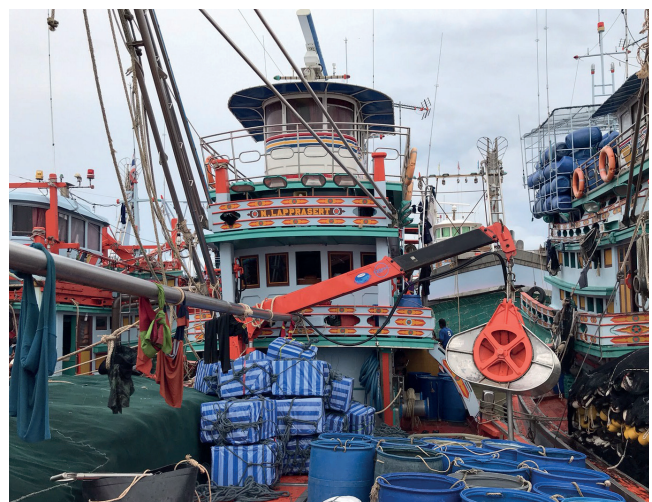
Picture 3: Power block and crane onboard the vessel (Photo: SEAFDEC)
